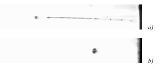
Figure 1. The jets of the standard ink (a) and polyacrylamide solution of concentration of 100 p.p.m. and molecular mass of 2,000,000 (b). Jet motion is from right to left. Longitudinal frame size corresponds to 2 mm. The flight time is 140  $\mu$ s.
